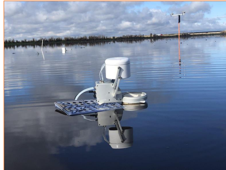
▲ Chambers on crates with long collars measuring flooded agriculture soils
